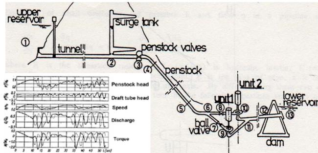
**Figure 1 Bajina Basta pumped-storage plant; two pump-turbines each 315 MW output and pump discharge 51 m<sup>3</sup>/s at speed 428.6 rpm; head 600 m. Low specific speed unstable “S” form four-quadrant curves are the source of severe transients even at one unit load rejection. Penstock pressure prevented to exceed designing pressure but water**
