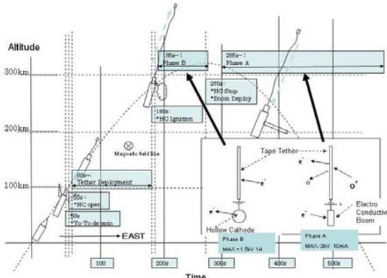
Figure 2: Experimental Sequence of the Sounding Rocket
