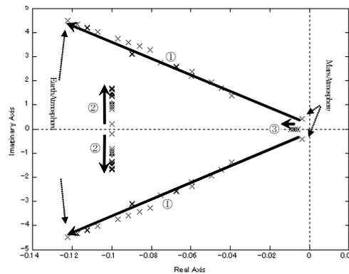
Figure 5: Root locus for the gravity acceleration from  $0.5G$  to  $1.5G$  (The air density  $1.2\text{g/m}^3$  and flight velocity  $0.5\text{m/s}$ )
