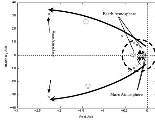
Figure 4: Root locus for the atmospheric density from  $0.01\text{kg/m}^3$  to  $1.0\text{kg/m}^3$  (gravity  $1G$ , and flight velocity  $0.5\text{m/s}$ )
