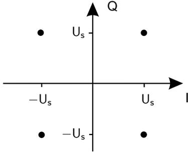
Fig. 6. Definition of the half-level transmit amplitude  $U_s$  for QPSK ( $M = 4$ )
