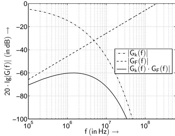
Fig. 3. Cable and FEXT coupling transfer functions for a cable length of  $l = 1.0 \text{ km}$  with  $K_F = 2.6248 \cdot 10^{-17} (\text{Hz}^2 \cdot \text{km})^{-1}$
