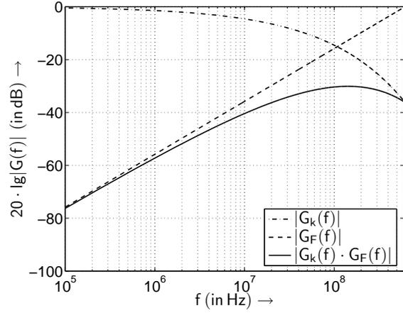
Fig. 2. Cable and FEXT coupling transfer functions for a cable length of  $l = 0.1 \text{ km}$  with  $K_F = 2.6248 \cdot 10^{-17} (\text{Hz}^2 \cdot \text{km})^{-1}$
