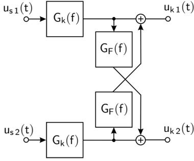
Fig. 4. MIMO cable transmission model system with FEXT ( $n = 2$ )
