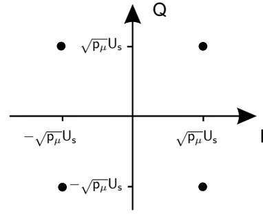
Fig. 7. QPSK constellation of the  $\mu$ th symbol after power allocation
