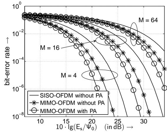
Fig. 10. BER comparison analyzing SISO-OFDM ( $n = 1$ ) and MIMO-OFDM ( $n = 10$ ,  $K_F = 10^{-13} \text{ (Hz}^2 \cdot \text{km)}^{-1}$ ) with and without PA for different QAM constellation sizes
