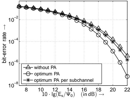
Fig. 9. BER comparison analyzing MIMO-OFDM ( $M = 4$ ,  $n = 10$ ,  $K_F = 10^{-13} \text{ (Hz}^2 \cdot \text{km)}^{-1}$ ) with and without PA
