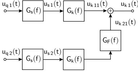
Fig. 1. Model of transmitter and cable with FEXT (example:  $N = 2$ )
