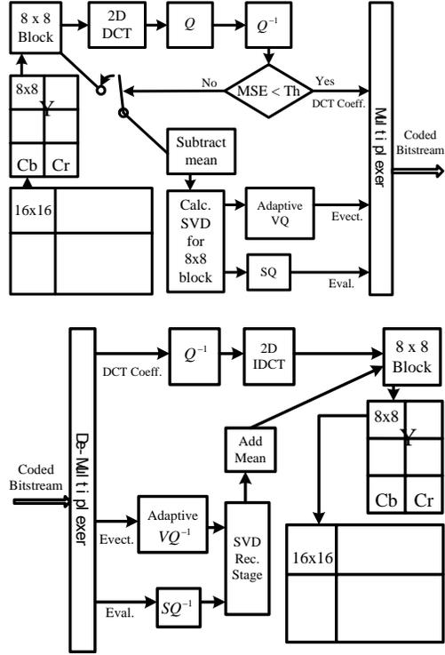
Fig.5. Block diagrams of HDCTSVD encoder and decoder.
