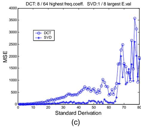
Fig.2. Motivation analysis. (a),(b),(c), performance comparison between DCT and SVD by taking the same ratio of coefficients.
